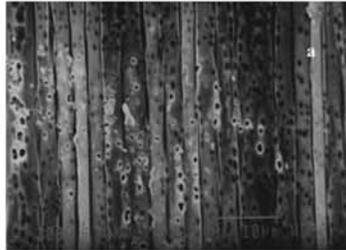
**Figure 3.** SEM photo of section of Si (100) sample treated by MPC in presence of normally orientated 480 mT magnetic field
