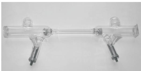
**Figure 1.** The glass discharge tube, with cylindrical indium plates, used in the experiment.
